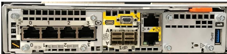
Figure 8. Embedded module with 10 GbE BASE-T 4-port card
