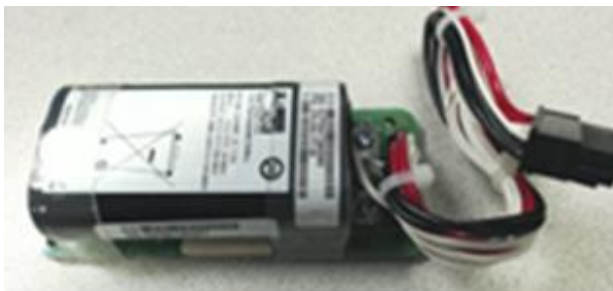
Figure 6. Battery backup unit
