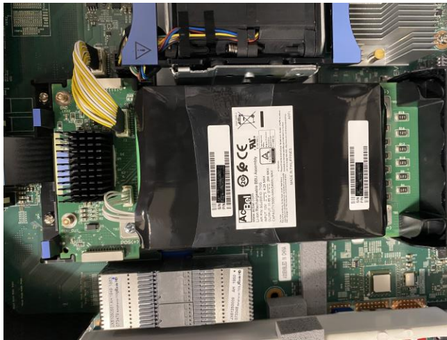
Figure 13. Battery backup unit
